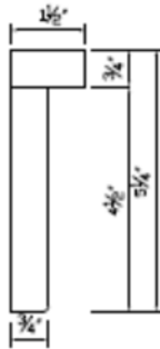
1/8" ROUNDED EDGE BOTTOM AND END EDGES CH 150
