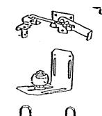
**ADJUSTABLE, OFFSET STAY ROLLER:** Tough, long-lasting Delrin guide wheel. Adjusts for doors up to 3-5/8" thick on center slot; up to 2-1/2" thick on outside slots. Bracket can be inverted for anchoring into concrete. Used on bottom of door.
