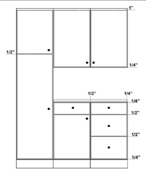
Vertical reveals between doors or drawers of connecting cabinets will be 1/2". Horizontal reveals between stacked drawers, between drawers and doors and between stacked doors will be 1/2". Reveals at the top of wall and tall cabinets will be 1" and the bottom will be 1/4". Reveals at the top and bottom of base, office and vanity cabinets will be 1/4".
