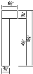
1/8" ROUNDED EDGE BOTTOM AND END EDGES CH 150
