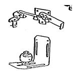
ADJUSTABLE, OFFSET STAY ROLLER: Tough, long-lasting Delrin guide wheel. Adjusts for doors up to 3-5/8" thick on center slot; up to 2-1/2" thick on outside slots. Bracket can be inverted for anchoring into concrete. Used on bottom of door.
