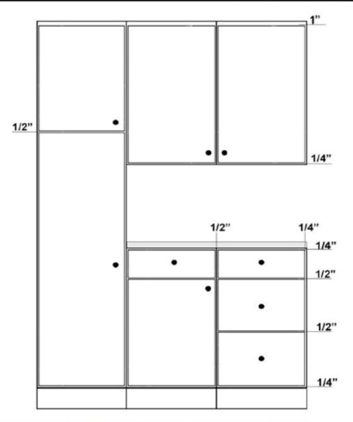
Vertical reveals between doors or drawers of connecting cabinets will be 1/2". Horizontal reveals between stacked drawers, between drawers and doors and between stacked doors will be 1/2". Reveals at the top of wall and tall cabinets will be 1" and the bottom will be 1/4". Reveals at the top and bottom of base, office and vanity cabinets will be 1/4".
