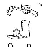
ADJUSTABLE, OFFSET STAY ROLLER: Tough, long-lasting Delrin guide wheel. Adjusts for doors up to 3-5/8" thick on center slot; up to 2-1/2" thick on outside slots. Bracket can be inverted for anchoring into concrete. Used on bottom of door.
