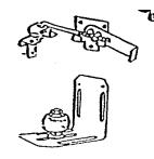
ADJUSTABLE, OFFSET STAY ROLLER: Tough, long-lasting Delrin guide wheel. Adjusts for doors up to 3-5/8" thick on center slot; up to 2-1/2" thick on outside slots. Bracket can be inverted for anchoring into concrete. Used on bottom of door.
